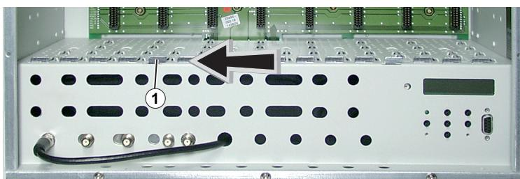
→ Slots 1 (digital module) and 2 (modulator module) are shown in the following figure. The open slot in between (without a contact strip on the board at the rear wall of the housing) is intended for an add-on module.
