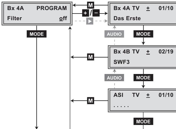
→ The following figure shows the "Setting the station filter" menu of channel strip "B".
