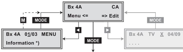
—> By pressing the **MODE** button you can skip the "Configuring the CA module" – "CA" menu and activate the "Setting the QAM modulation" – "QAM" menu (page 31).
