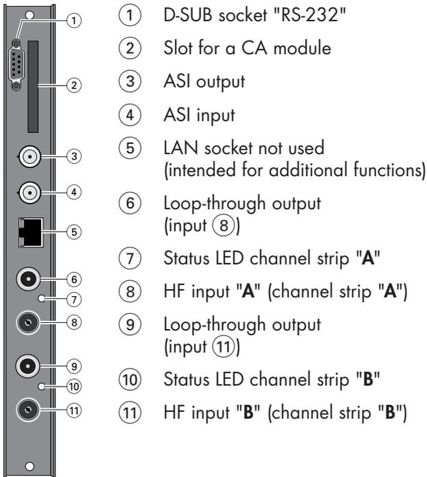
The operating software of the cassette can be updated via the 9-pin D-SUB socket "RS-232" using a PC or notebook and the software "**BE-Flash**". You can find the current operating software on the website "[www.gss.de](http://www.gss.de)".
