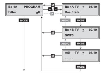
$\longrightarrow$  The following figure shows the "Station filter" menu of channel strip " ${f B}$ ".
