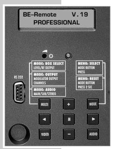
Setting up of the modulator box is exclusively effected via the keys of the Headend station's control unit.
